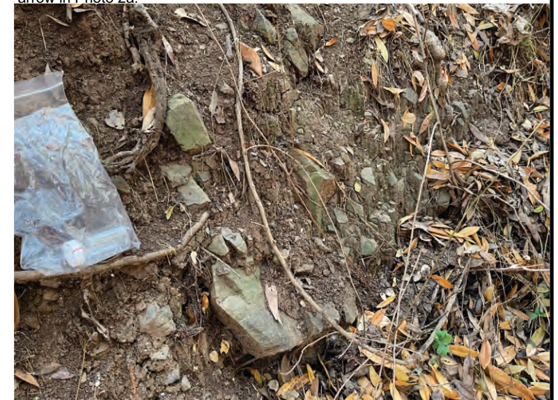
Photo 4b. Exposure of closely jointed graywacke in bank of the dry channel about 100 feet downstream from the sample location in Photo 4a.
