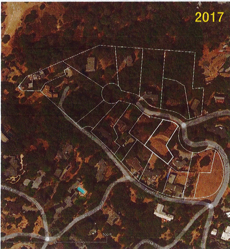
Figure 2. Historical aerial photos show increased home building, tree removal, and landsliding, Los Cerros Rd and Palomar Dr area, San Mateo County, CA. Major landsliding documented during wet years 2017, 1982-83, and 1950s.
