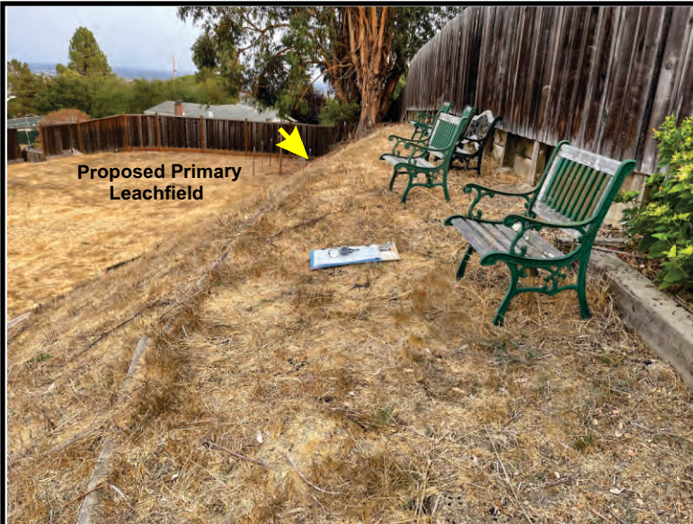
Photo 1a. Southeast view along top of cut slope along southwest margin of Site. Inferred 18% northeast facing native slope extends across property line fence.
