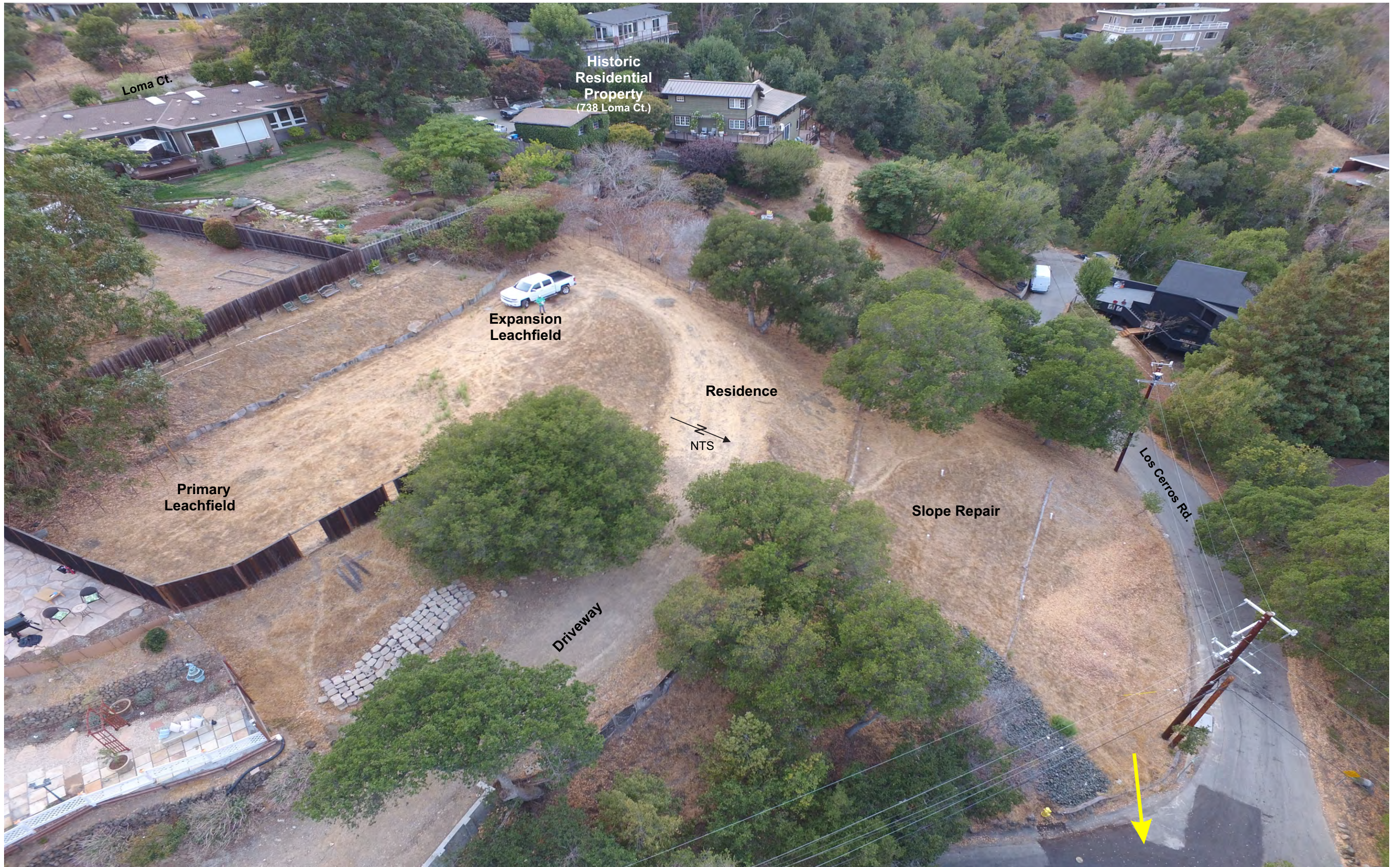
Figure 1. Westerly aerial drone view of proposed residential development area and adjoining area (09/25/2021). Arrow in lower left of view is recent replacement of Cal Water Service main that caused seepage onto Palomar Drive in winter of 2020.
