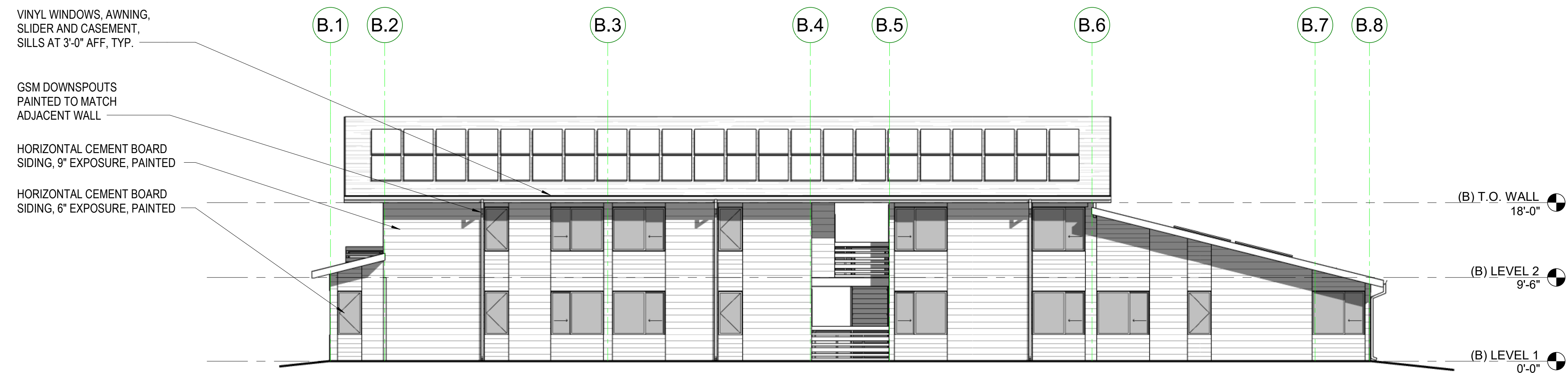
BUILDING TYPE B - WEST ELEVATION ② 1/8" = 1'-0"
