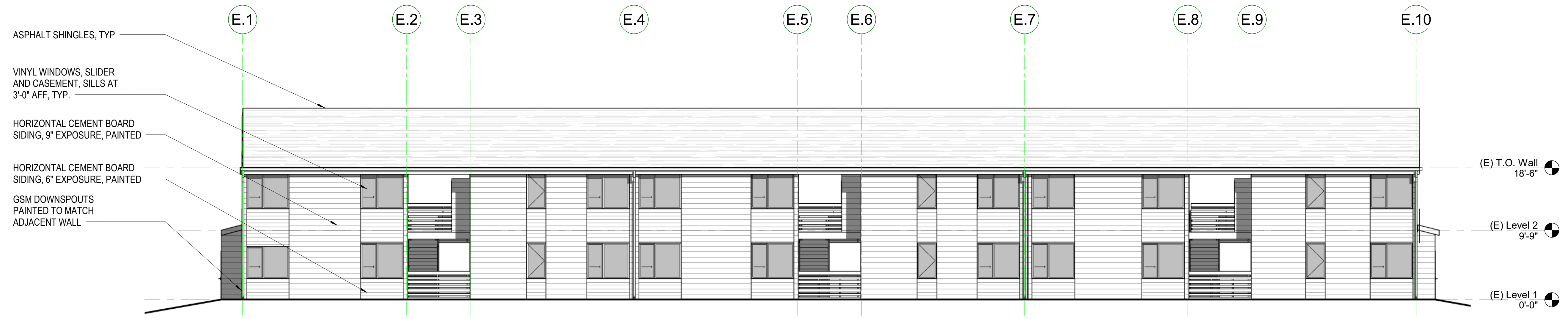
BUILDING TYPE E - EAST ELEVATION 1/8" = 1'-0" 1
